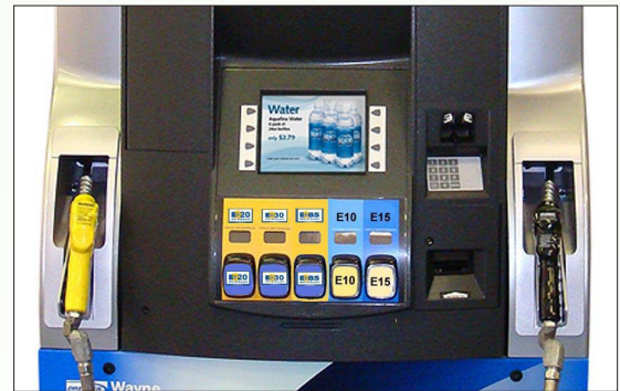
DIAGRAM 2. E 10 and E15 must be sold from the same hose with proper labeling. Proper labeling not affixed.
